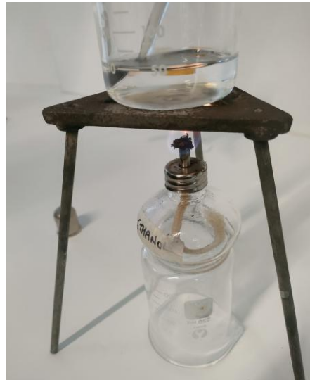
Figure 2 – Placing the spirit burner closer to the water.
