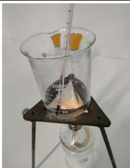
Figure 1 – the setup of the spirit burner and beaker.
